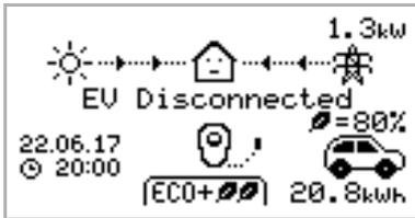
The EV is not connected to zappi
