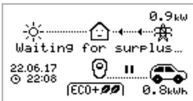
zappi is waiting for sufficient surplus power from the microgeneration system. This screen will be shown in ECO+ mode as it's only in this mode that charging will stop if there is not enough surplus power.
