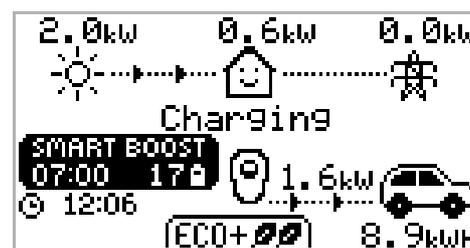
3. zappi will then test the EV for a few seconds, to determine the maximum charge rate.
